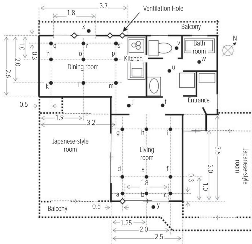
Figure 1. Arrangement of the sampling points (a to y, solid circle) in the room layout. The midair squares (4 points, near the windows) represent ventilation holes. The unit of length is the meter.
