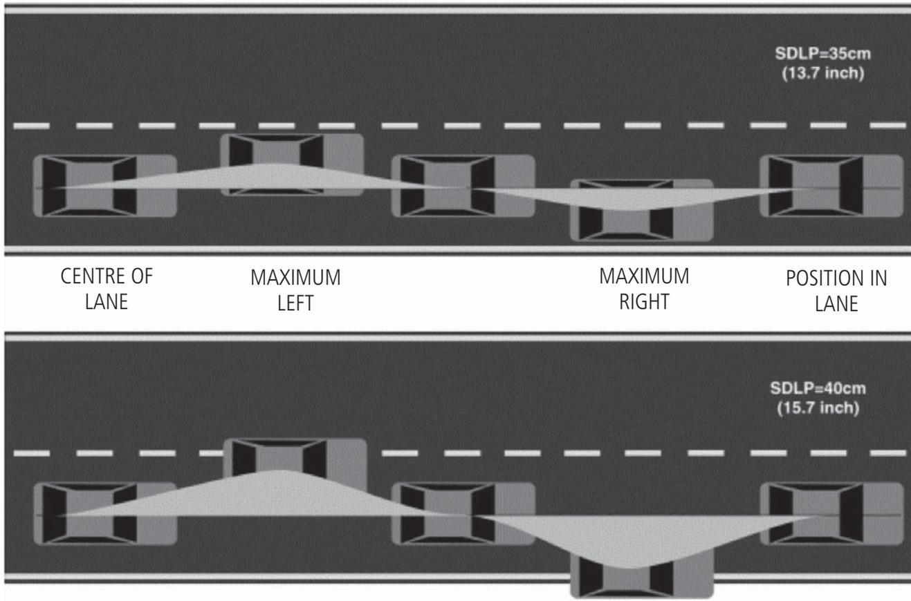
**Figure 2.** In the standardized highway driving test in healthy volunteers, the principal parameter measured is the ability to keep the vehicle in the centre of the lane, or the standard deviation from the lateral position in cm (SDLP) [46]
